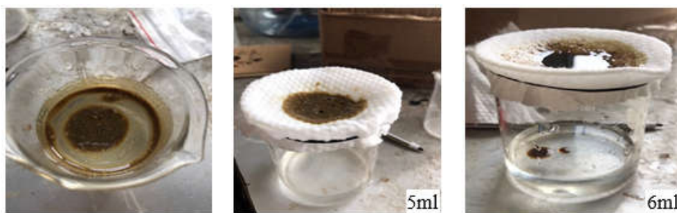
Figure 7. Experimenting on the waste oil absorption capability of spongy nanocomposites based on \text{Al}_2\text{O}_3 hybridizing with stearic acid
